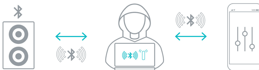
Figure 5// Architecture of a MitM attack taking place between a Bluetooth device and the app used to control it
